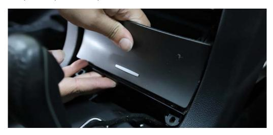
Bottom compartment with closing lid The clips are on the rear as shown
