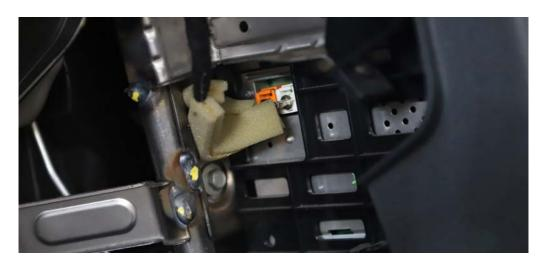
**Disconnect Antenna**Press down on the top of the connector to remove from the headunit
