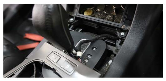
**Bottom compartment with closing lid**Remove the 2x screws holding in the bottom compartment
